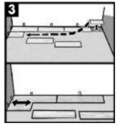
8. Start the third row with the plank cat at 1/3 of a length (16"). Again the remaining piece can be used at the opposite end of the row, if the layout of the room permits.
